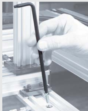
As the clamping action is purely mechanical, MagicSpring® also gets a firm grip on TORX® or TORX PLUS® screws made of aluminium, stainless steel, plastic and titanium.
