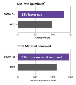
'Results based on an automated, 11 minute test on 1018 steel using a 3M<sup>™</sup> Cubitron<sup>™</sup> II Fibre Disc 982CX Pro, 7", grade 36+ and 3M<sup>™</sup> Disc Pad Face Plate Ribbed 80514 on a servo motor.
