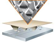
Conventional ceramic abrasive grain tends to "plow" through the metal, causing heat to build up in the workpiece and the abrasive – resulting in a slower cut and shorter abrasive life.
