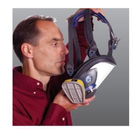
Fully loosen all six head straps. Hold the front of the facepiece with one hand and the straps/comfort cradle away from the facepiece with the other hand, creating an opening for the head. Pull the respirator assembly down over the head. Place the nose in the nose cup and chin in the chin cup area then press the facepiece firmly and evenly against the face.
