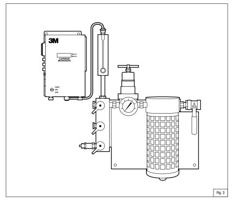
Assembled  $3M^{\scriptscriptstyle TM}$  Retrofit Kit W-2808/37027 attached to  $3M^{\scriptscriptstyle TM}$  Compressed Air Filter and Regulator Panel W-2806/07006 (sold separately).
