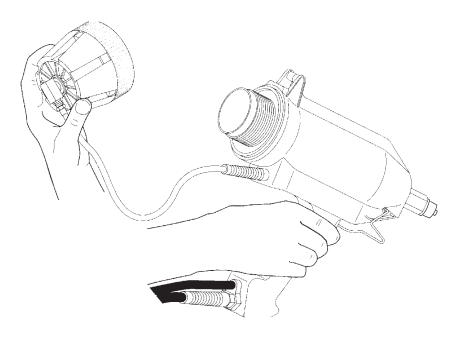
3. Replace and tighten end cap, turning it in a clockwise direction. Increases air pressure to approximately 80 psi. If adhesive begins to flow, readjust to desired pressure. If there is still no or low-adhesive flow, continue to next step.
