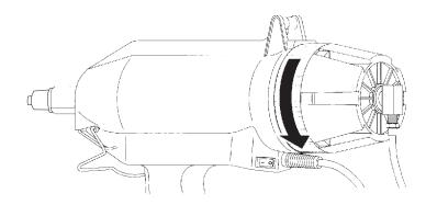
3. Remove empty cartridge with attached nozzle assembly from applicator and discard.
