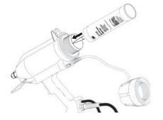
8. Tighten applicator end cap clockwise to ensure a positive seal. Allow cartridge to warm for a minimum of 35 minutes. Follow "Dispensing" procedure for trouble free operation.
