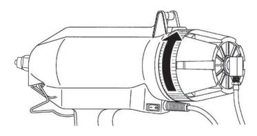
2. Remove end cap by rotating end cap counterclockwise.
