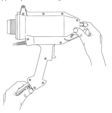
11. Hold the trigger in the upper housing and lift off.
