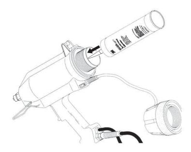
6. Adjust the Shroud: With a Scotch-Weld PUR Easy adhesive cartridge and Disposable Nozzle loaded in the applicator, insert Nozzle Shroud (A) into Nozzle Warmer (B) allowing Approximately 1/16" of the Disposable Nozzle protruding as shown and tighten set-screw (C) to secure
