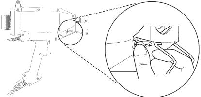
Remove end cap by turning counterclockwise.
