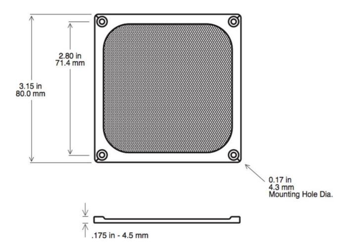
Aluminium/stainless filters offer high levels of air passage while efficiently filtering contaminants and shielding EMI/RFI.
