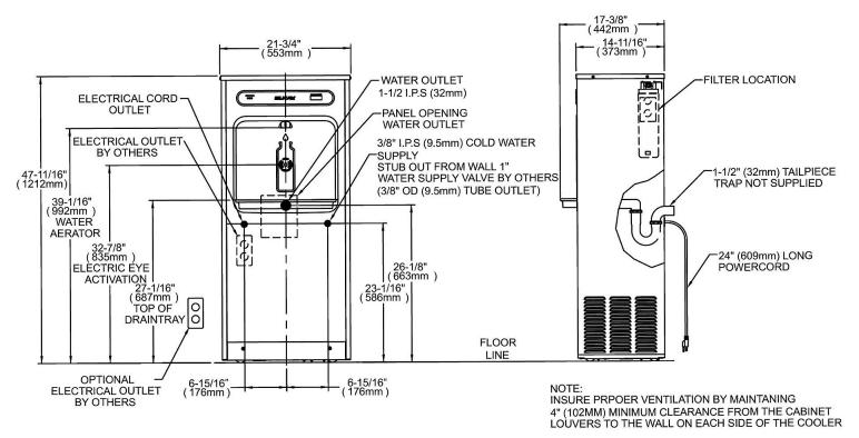
NEW INSTALLATIONS MUST USE GROUND FAULT CIRCUIT INTRUPTER (GFCI) IT IS HIGHLY RECOMMENDED THAT THE CIRCUIT BE DEDICATED AND THE LOAD PROTACTION BE SIZED FOR 20 AMPS
