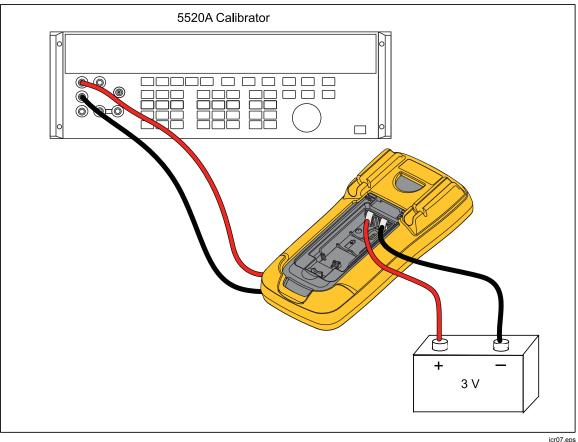
Figure 4. Calibration Connections
