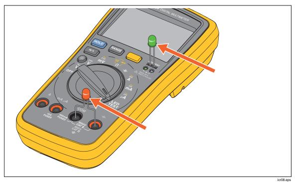
Figure 2. LED Test
