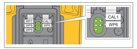
Figure 7. Calibration Adjustment 18B+
