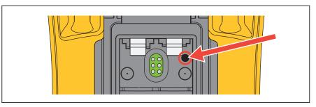
Figure 6. Temperature Adjustment for 17B+
