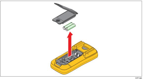
Figure 1. Remove the battery
