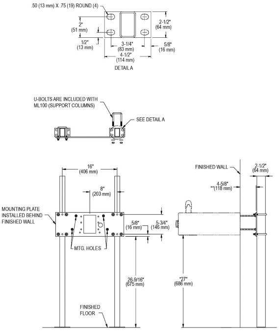
\* ADA REQUIREMENT \*\* WITH STANDARD STUD LENGTH OF 6 INCHES. NOTE - AFTER INSTALLATION, U-BOLTS AND THREADED RODS MAY NEED TO BE TRIMMED.
